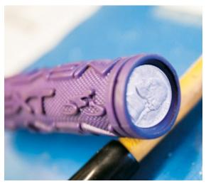
Many riders put a coin in the bottom of their grips to prevent the bar from cutting through the rubber.
