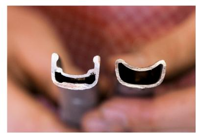
Cross-section of rims: hooked, left; tubular, right
