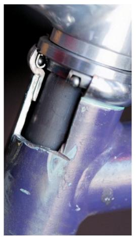
Cutaway view of head tube and headset assembly
