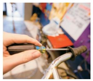
A long, thin screwdriver is great for opening up a space to spray soapy water when removing grips, if necessary.
