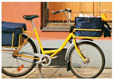
For transporting a lot of goods on a regular basis, consider front and back brackets for carrying substantial loads, such as on this mail delivery bike.
