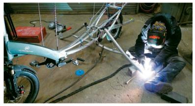
Metalworker by day, bicycle customizer by night. Jay Broemmel welds a mounting point for the retractable outrigger wheels on Fossil Fool's tall bike, El Arbol, shown below.
