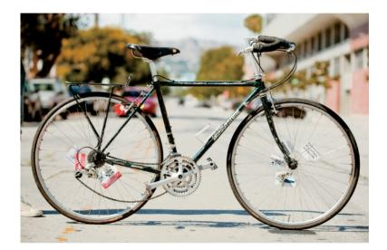
Seat tube angle is measured against the ground; a 90-degree seat tube would be completely vertical. The greater the seat tube angle, the closer it is to vertical, and the more it is considered to be an "aggressive" geometry. This is because a more vertical seat tube moves the rider farther forward over the pedals, which allows for great power in the downstroke, but is less comfortable.
