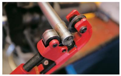
Don't over-tighten the pipe cutter; they are easy to break.
