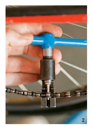
**2.** Slowly twist the handle to drive the pin into the chain, slowly pushing out the pin from inside the chain.
