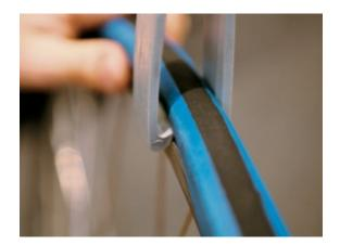
**5.** Once your bead is back on, fill the tire to the desired pressure, paying attention for bulges; if the wire bead isn't set properly, a section of the tire might bulge out. Inspect all the way around once you have filled your tire to ensure that the bead is properly seated on the rim. If it is not, your tire might not be compatible with your rim.
