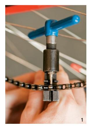
**1.** Take the chain into the chain breaker and mount the rollers on the set of pins closest to the handle.
