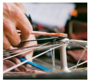
Using a flat wrench to hold your cone nut in position, set the tension on the system using either a flat or normal wrench on the lock nut. Be sure to check the place with the wheel upright; it often changes the way the axle feels as opposed to being on its side.
