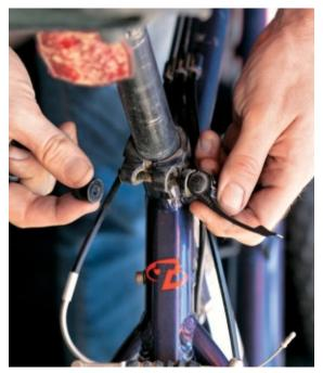
Remove the quick-release bolt that comes with most bikes.
