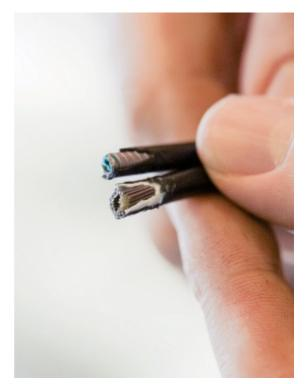
brake cable; bottom: shifter cable
