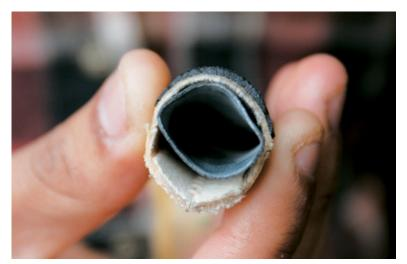
Cross-section of a tubular tire
