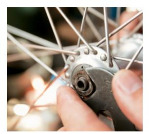
Remove the cone nuts using flat wrenches.
