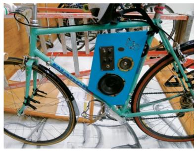
A bicycle sound system in the front triangle, complete with input for an MP3 player or electric guitar, and knobs for volume and tone.
