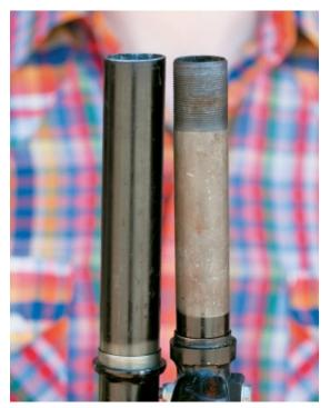
Threaded and threadless steerer tubes
