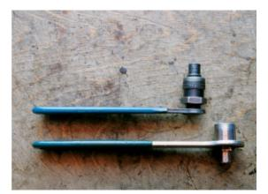
Crank puller/crank bolt wrench
