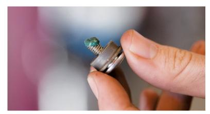
Crank bolt with grease
