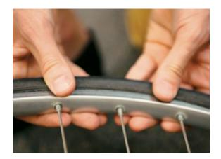
The final bit may be challenging, but do not use your tire levers: you can puncture the tube by doing so. Standard thumb strength, and working patiently, is generally enough.
