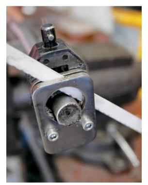
Attaching a guide helps you keep your saw cut straight and level.
