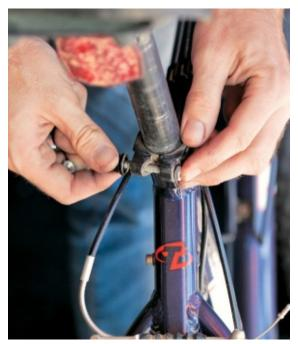
Replace it with a normal bolt from a hardware store; often you can re-use the original quick-release nut.
