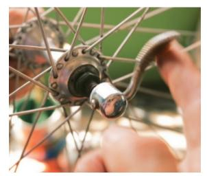
Removing the quick-release skewer
