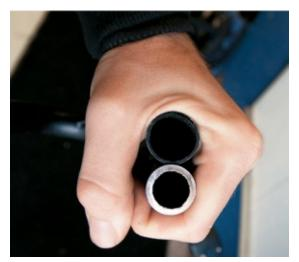
Road bars have a thicker tube diameter than mountain bars, while in this case the mountain bar has thicker tube walls.
