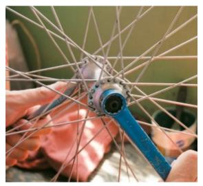
Remove the outside locknuts using regular wrenches.
