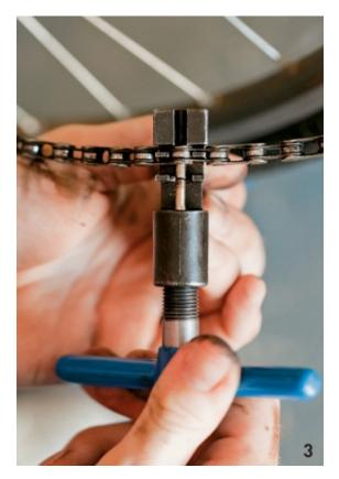
**3.** Stop before removing the pin all the way from the chain; the goal is to leave the pin resting in the outside plate of the chain, so that you can later reinsert it and reassemble the chain. It's not a disaster if you push the pin all the way through, but it's best avoided.
