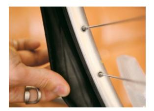
Once you have the wheel off the frame, examine the outside of the tire for any indication of what might have created your flat. Obvious culprits could be giant thorns, chunks of glass, or rips in the sidewall of the tire.
