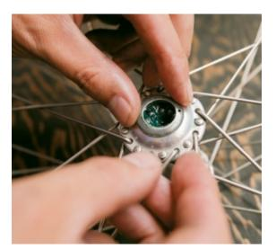
Replace the dust cap if necessary.
