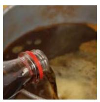
I poured the coke all over my pan. There is some chemical reaction that quickly gets the rust off. This is mostly surface rust, so I could wipe it off after a few minutes. For deeper rust you have to let it sit for longer.
