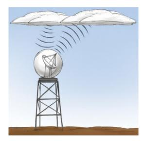
Radio transmitters use microwaves to detect precipitation intensity and locations.
