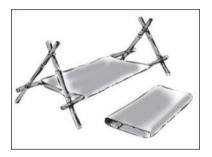
An A-frame pole bed is usually supported by two larger trees. The tension in the bed—which can be made from plastic feed sacks—holds the bedding poles in place.
