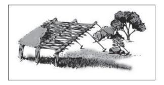
Before bricks, most houses were constructed with a timber frame supporting wattle and daub—a lattice-work of sticks caked with mud. The same method can be used to build shelters on plains and grasslands.
