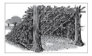
One of the best shelters to build is a simple lean-to. Note the wind direction and then site your frame accordingly, using available branches to construct it. Cover the frame with foliage thick enough to stop the wind and rain, and then cover the sides to give extra protection.
