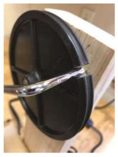
Step 13 Cut notch in pulley and sit popper crank inside.
