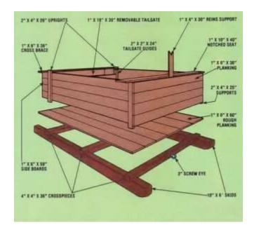
Here In Quebec, we've found our easy-to-build horse-drawn sled to be just about the ideal device to handle the kind of haulin' chores that crop up almost daily on a farm. And–since most of the materials needed to **construct** the simple freight carrier are probably already around just waitin' to be used–you can put the versatile sled to work on **your** homestead for next to nothing!
