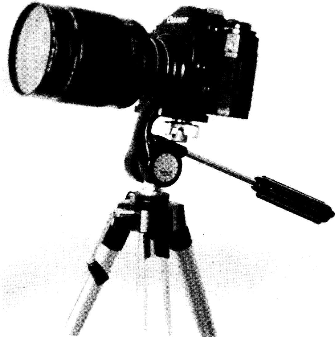
500 mm catadioptric lens w/2X multiplier attached, a deadly combination of camera and lens for long-range work on a budget, but with strict limitations. See text.
