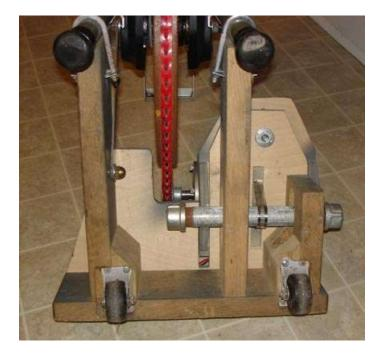
Step 4: Making the generator cradle Cut two pieces of 1/2" plywood to fit the diameter of your generator. Cut slots in the cradle base by drilling a series of small holes close together. An 1/8" router bit could also be used to cut a slot.
