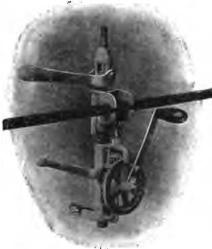
FIG. 15. DRILLING MACHINE FOR THE INSTALLATION OF THE SKINNER SYSTEM OF IRRIGATION
